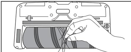
Place motorized floor nozzle upside down. Use fingers to remove clog or debris. Do not use scissors or knife to cut strings and threads.
