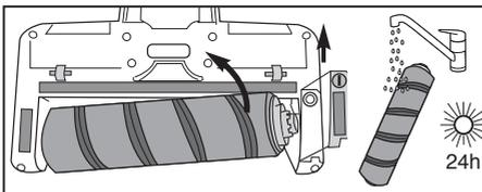
Remove retainer clip and lift out brush roll to clean and remove debris. Brush roll is washable. Roll in a towel to absorb water; dry THOROUGHLY before reassembling.
