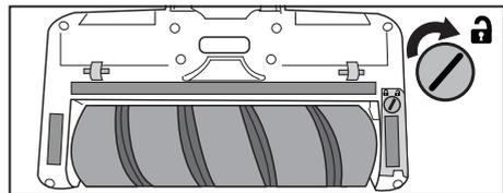
If debris cannot be removed easily, remove retainer clip to access brush roll. Using flathead screwdriver or coin, turn screw to the 'unlock' position.
