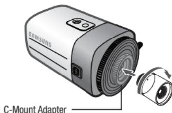
3. After combining the lens, adjust the focus.
