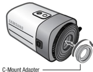
2. Turn the C-Mount lens clockwise to install it.
