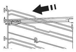
**4.** To secure the guide, press the lower portion of the clip firmly against the shelf guide. Make sure that the runners can move freely.
