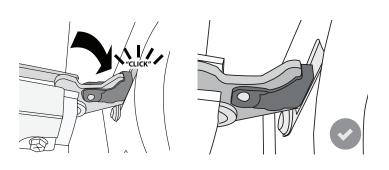
**6.** Try closing the door and check to make sure that it lines up with the control panel. If it does not, repeat the steps above: the door could become damaged if it does not work properly.
