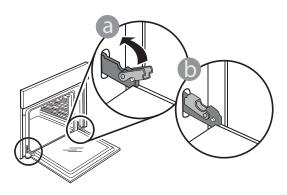
**5.** Apply gentle pressure to check that the catches are in the correct position.
