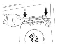
**4.** To reposition the heating element, lift it up, pulling it slightly towards you, be sure it comes to rest on the lateral supports.
