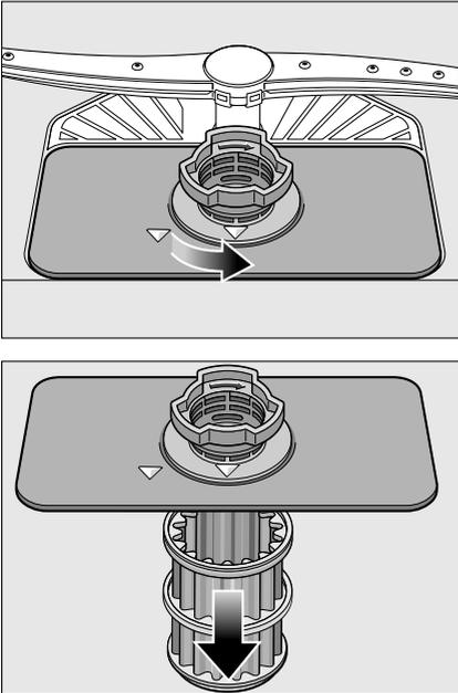
3. Remove any residue and clean filters under running water.
