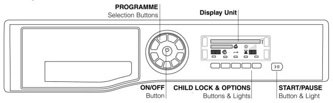
The **ON/OFF** button 1 - if pressed when the dryer is running: If the display shows TURNING OFF the dryer stops. If the display shows PRESS AND HOLD hold the botton and the display counts down 3, 2, 1 and then stops.
