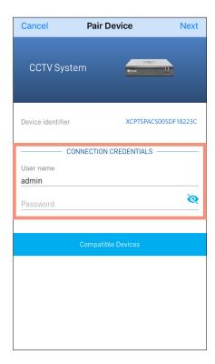
In the **Username** field, enter "admin". In the **Password** field, enter the password of your CCTV system which is the same password you use to unlock the system menu locally. This is normally the password that you created when setting up your DVR or NVR for the first time using the integrated Startup Wizard.
