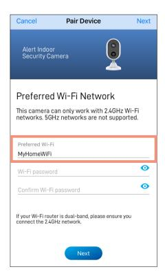
The Wi-Fi network name field is auto-filled with the Wi-Fi network that your phone is currently using. Your camera will join this Wi-Fi network by default.
