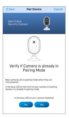
Check if the LED indicator of your camera is blinking blue slowly as shown. If so, your camera is already in pairing mode (i.e., the camera's hotspot is activated temporarily) and ready to pair. Tap the **Yes** button.
