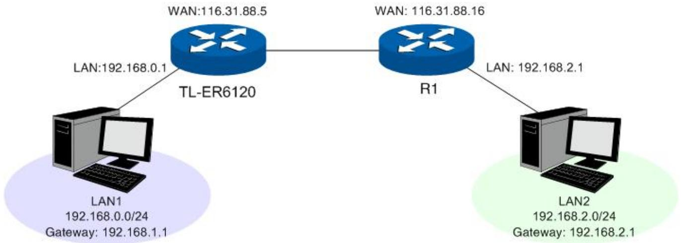
If the LAN port of TL-ER6120 (with Non-NAT or Classic system mode) is connected to LAN1 with subnet of 192.168.0.0/24, while the LAN port of another Router R1 is connected to LAN2 with network of 192.168.2.0/24. Meanwhile, the WAN ports of the two routers are interconnected and within the same network. Now a host under TL-ER6120 and within network of LAN1 desires to communicate with the host within network of LAN2.
