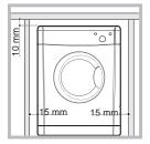
If you are going to install the appliance under a work counter be sure to leave a 10mm space between the top and any other objects on or above the machine and a 15mm space between the sides and any kitchen units or
