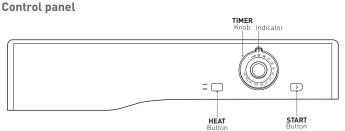
The **HEAT** button selects drying temperature. OUT: LOW heat IN: HIGH heat. The **TIMER** knob: the **0** position swithes off the dryer.
