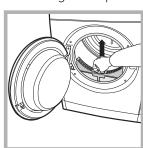
Check the vent tube and any permanent venting fixture to make sure that there has been no accumulation of fluff or lint. Remove lint that collects around the filter and the outlet vents.
