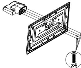
2. Place the stand(s) on the stand mounting pattern(s) on the rear side of the TV.
