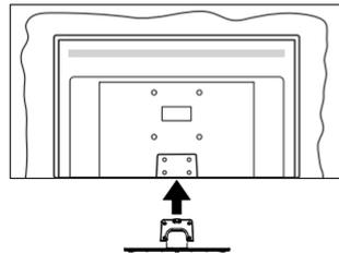
3. Insert the screws (M4 x 12) provided and tighten them gently until the stand is properly fitted.
