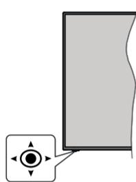
This TV has a joystick as shown in the above drawing. It allows you to control the Volume / Programme / Source and Turn Off-On functions of the TV.
