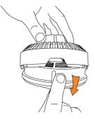
Remove the post-motor filter from the filter cover.
