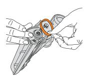
Clean any debris from the spindle. Place the new belt onto the spindle and line up the teeth on the belt with the teeth on the cog. Slide the belt into place.
