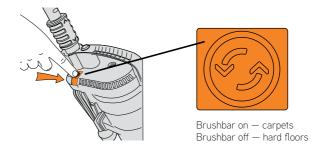
**NOTE:** The brushbar will not spin until the machine is reclined.
