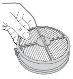
Check the post-motor filter for discolouration.
