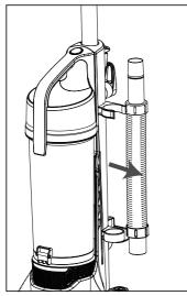
2. Remove the tube (2) from the main body by pushing the handle release button (10).
