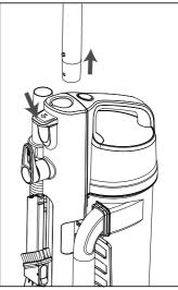
3. Assemble the hande onto the hose.4. Attach the tube onto the hose.
