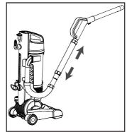
5. Assemble the 2in1 accessory (12) onto the tube (2).
