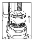
2. Remove the post motor filter by lifting it.
