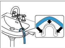
Fix and secure the water outlet hose with an elbow → Page 27.
