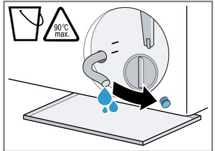
8. Firmly press on the sealing cap.
