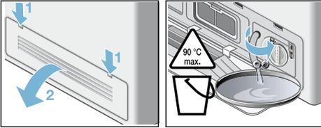
5. Remove the cover flap, draining the washing water into a suitable container. Press on the cover flap and insert the drainage hose into the holder.
