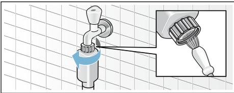
6. Clean the filter on the back of the appliance:
