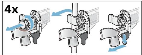
5. Insert the covers. Lock firmly by pressing on the locking hook. Insert the hose holder.
