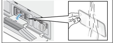
4. Rinse fluff off the air filter using a brush under running water.
