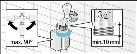
2. Carefully turn on the tap and check that the connection points are not leaking.
