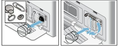
8. Close the service flap. If required, engage the disengaged service flap beforehand.
