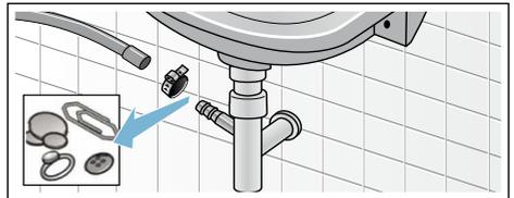
4. Re-attach the drainage hose and secure the connection point with the hose clip.
