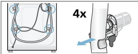
4. Take the power cord out of the holders. Remove the sleeves.
