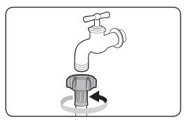
**7.** If you are using a screw type of water tap, use the provided screw-type adaptor to connect to the water tap as shown.
