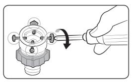
**2.** Use a Philips screwdriver to loosen four screws on the adaptor.
