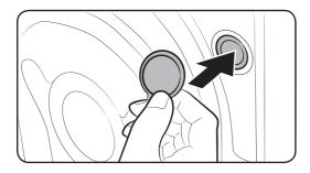
**2.** Fill the holes with the supplied plastic bolt caps.
