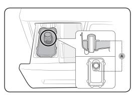
First insert the provided liquid container in the II main-wash compartment. Then, apply liquid detergent to the container below the marked max line (A).
