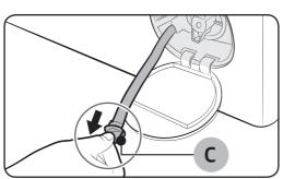
**4.** While holding the end of the drain tube, open the tube cap (C).
