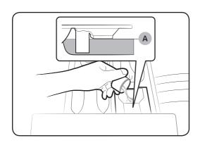
**3.** Apply fabric softener to the **softener** compartment. Do not exceed the max line (A).
