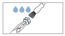
Connect the hose and check for leaks.
