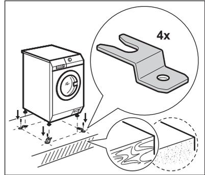
If you install the appliance on a concrete base, please make sure to order the correct anchoring kit.
