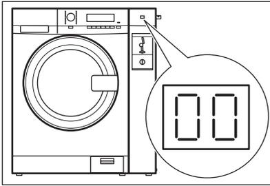
Insert correct amount of coins. When inserting coins, the display on the coin meter counts down to "00" (then it shows **--** or **00**) and the appliance is ready to start.
