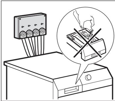
The liquid detergent can be loaded automatically from an external dispenser. Read carefully the instructions supplied with the accessory.
