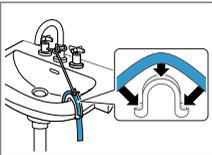
Fix and secure the water outlet hose with an elbow → Page 29.
