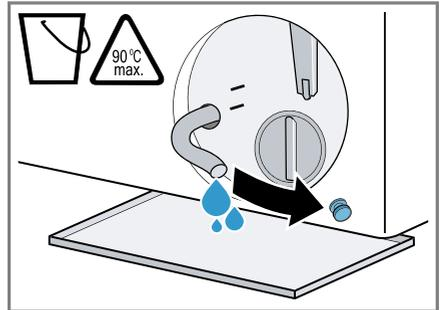
8. Firmly press on the sealing cap.
