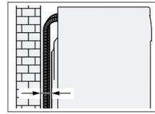
Do not trap the hoses between the wall and the appliance.
