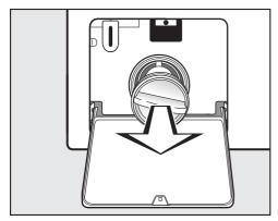
Remove the drain filter completely.
