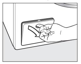
Open the drain pump access panel.
