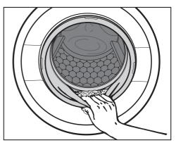
Check the folds in the door seal for any small articles, e.g. buttons, which might be lodged there.
