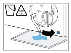
9. Firmly press on the sealing cap.
