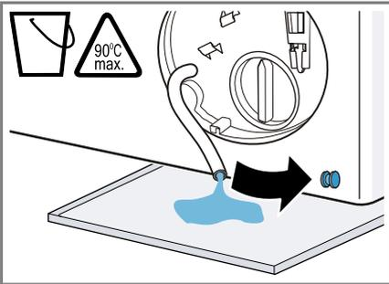
9. Firmly press on the sealing cap.
