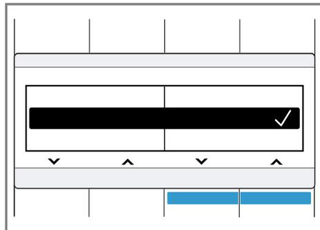
If a setting is activated, the display shows ✓. The selection does not need to be confirmed again. The sub-menu closes automatically after a few seconds.
