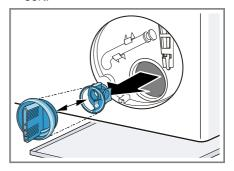
**2.** Clean the inside and the thread on the pump cap and pump housing.
