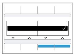
If a setting is activated, the display shows  $\checkmark$ . The selection does not need to be confirmed again. The sub-menu closes automatically after a few seconds.
