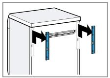
Undo and remove the screws in the horizontal transport strut using a T20 screwdriver.
