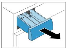
**2.** Press down on the insert and remove the detergent drawer.
