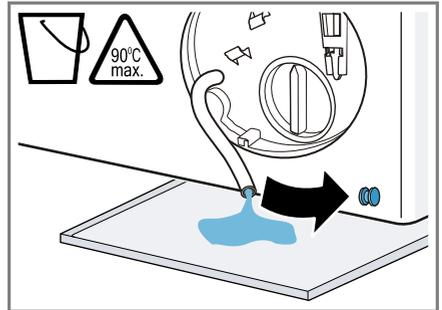
9. Firmly press on the sealing cap.
