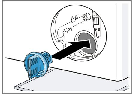
5. Screw on the pump cap.
