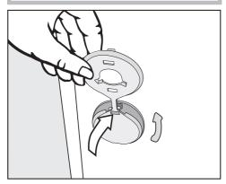
Fit the stoppers onto the two holes.
