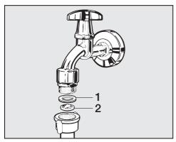
Remove the rubber seal 1 from the recess.
