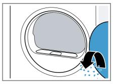
3. Remove the two-part fluff filter.
