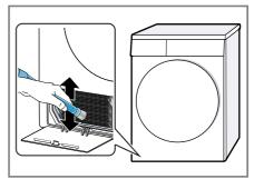
Ensure that you vacuum the fins from top to bottom so that they do not become deformed or damaged. 4. Clean the opening with a soft, damp cloth.
