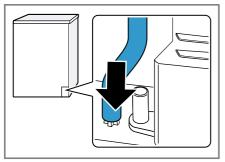
**3.** Push the water drain hose as far as it will go into the connecting piece.
