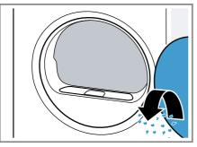
3. Remove the two-part fluff filter.
