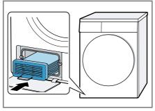
Ensure that the heat exchanger is inserted with its handle pointing downwards.
