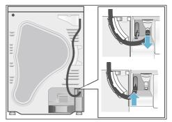
4. Take the drain hose from the accessories and secure it to the free connecting piece.
