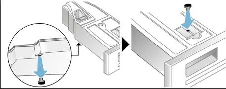
8. Pull the filter out of the lock-in slot and place it into the recess in the top of the condensation container.
