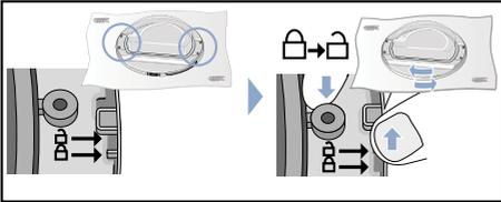
7. Now lift the dryer door from the door ring. Rotate the dryer door and place it back onto the door ring in the corresponding place.
