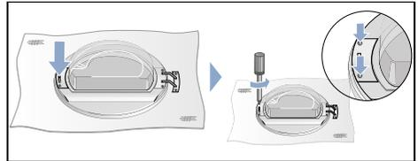
10. Remove the cover from the door lock on the dryer and place it to one side.
