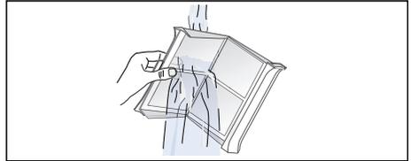
7. Dry the fluff filter, close it and reinsert the two-part fluff filter.
