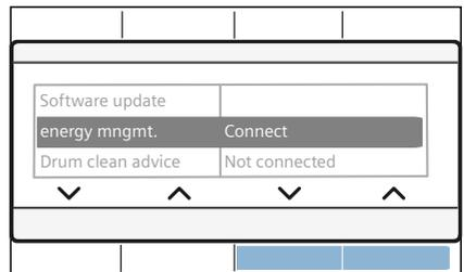
Your appliance now attempts to connect to the smart energy system (energy manager). If the appliance has connected successfully, **Connected** ✓ appears in the display.
