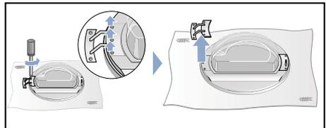
5. Remove the screws from the door handle on the dryer door and remove the door handle.
