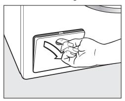
■ Open the drain pump access panel.
