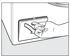
■ Open the drain pump access panel.
