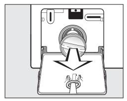
■ Remove the drain filter completely.
