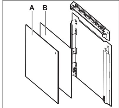
Make sure that you install the middle panel of glass in the seats correctly.
