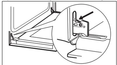
2. Lift and turn the levers fully on both hinges.
