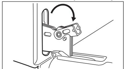
3. Close the oven door halfway to the first opening position. Then lift and pull forward and remove the door from its seat.
