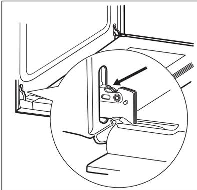
2. Lift and turn the levers fully on both hinges.
