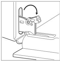
3. Close the oven door halfway to the first opening position. Then lift and pull forward and remove the door from its seat.
