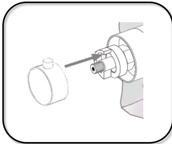
Fit temperature control handle to thermostat, ensuring the stop pin inside the handle, is located against the top of the stop ring.
