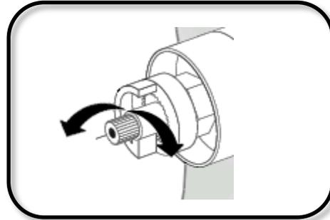
Pull the handle from the mixer. DO NOT remove the plastic stop ring.
