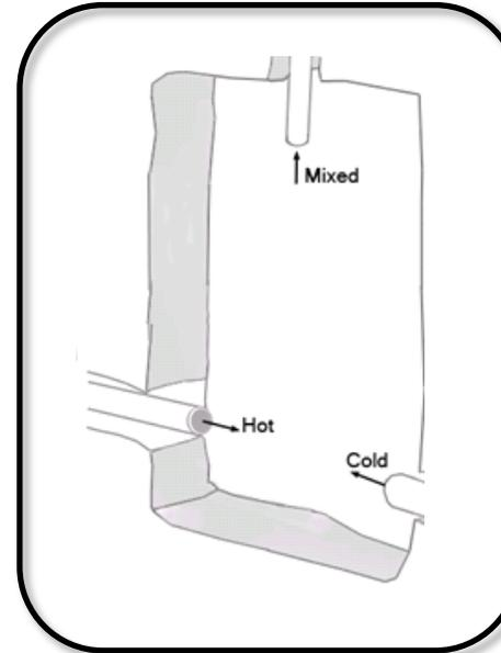
Prepare pipes in wall to connect to shower, with cold on the right.
