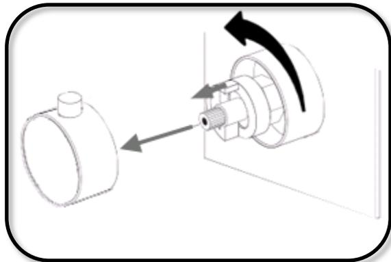
Using a spanner remove the thermostatic cartridge.
