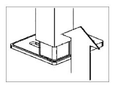
Set the frame so the top bar of the frame is 820mm above the finished floor level.
