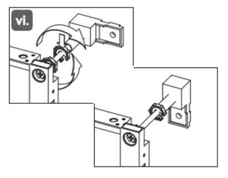
**Step 6**Place the two Bolt Location Blocks (k) into either side of the top frame profile.
