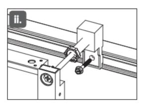
Using a pencil, mark through the two holes in the Wall Fixing Feet (J) the fixing hole positions.
