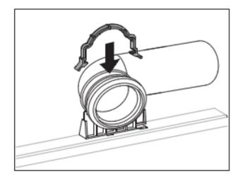
**Step 10**To install the 90° Pan Connector. Offer the soil pipe to the clamp and secure using the clamp.
