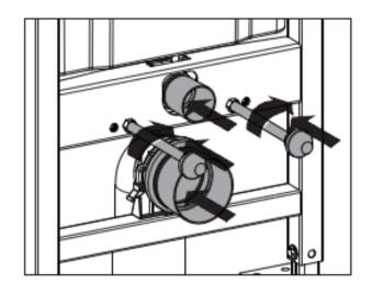
Connect the Debris Stopper for Flush Pipe Extension (U) and Debris Stopper for Soil Pipe Extension (S).
