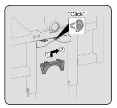
Ensure the soil pipe clamp is secure.
