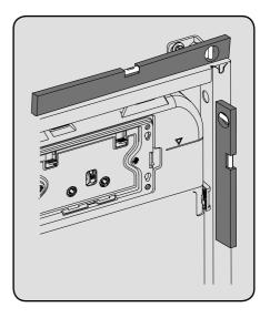
Step 4 Check the frame for level.
