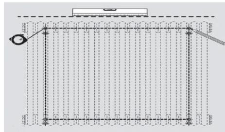
2. Using the drill and 8mm drill bit, drill into the marked positions then insert the wall plugs and tap flush to the finished wall surface.
