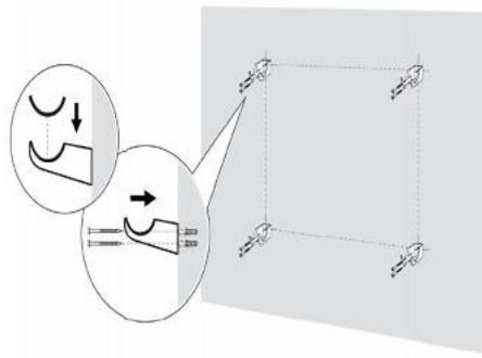
4. Once all brackets are secure, hang the radiator until fixed firmly into place and adjust so that the radiator aligns with the pipework.
