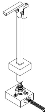
Fix the shower hose into the handset and fit the handset into the handset holder.
