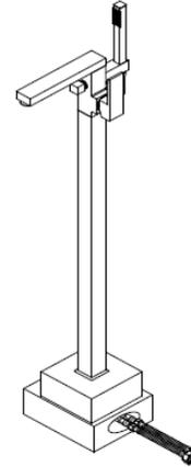
\*\*\* A recess is required with size 35(L)x35(W)x53(D)mm to fit the base foot.
