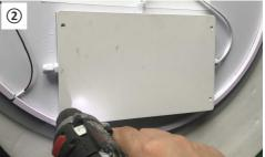
Unscrew the backboard and remove it.
