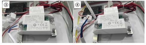
Remove the wires at both ends of the led driver. Unscrew the led driver base.
