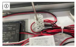
Loosen screw of led wire connecting terminal, remove the led wire.
