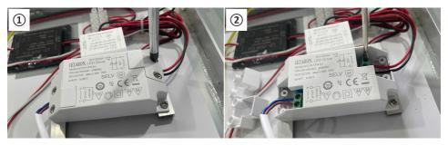
Unscrew both ends of the led driver cover.
