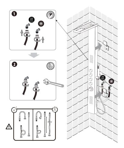
Fit the seal into the nut end of the shower hose and connect the nut to the outlet on the hand shower holder and tighten, if using a spanner, place a cloth around the nut to prevent damage.
