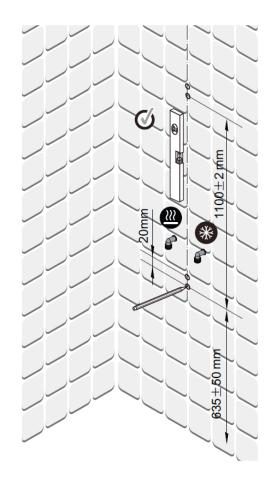
If drilling into tile, it is recommended to tape the wall to prevent the drill from slipping.
