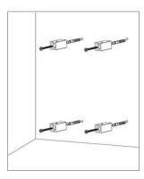
5. Next, proceed to fix the rail brackets to the rear of the radiator, screw these into place and tighten by hand.
