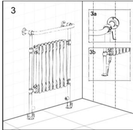
4. Insert the air vent in the top of the radiator, (add a little sealer tape to secure) and tighten, be sure not to overtighten then fit the radiator valves to the pipework and connect to the radiator valve tail and tighten all connections.
