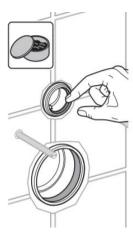
4. Connect the flush pipe and pan connector to the frame ready for connection to the toilet pan as shown, then screw the female threaded connectors (fixing bolts) onto the threaded bars so that the cut out aligns with the fixing hole in the toilet pan.
