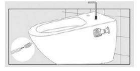
10. Once the installation is completed, a flush and leak test should be carried out and once it has been commissioned, the toilet can be sealed around the edge to finish.
