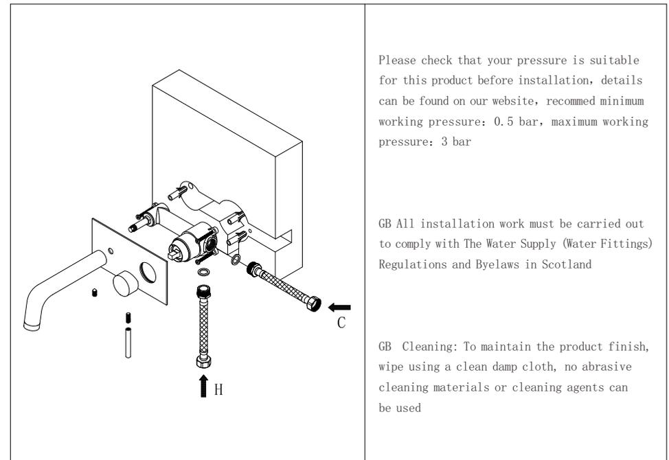
Please check that your pressure is suitable for this product before installation, details can be found on our website, recommended minimum working pressure: 0.5 bar, maximum working pressure: 3 bar
