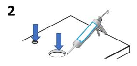
Seal the inside/exposed edge after cutting to prevent water/moisture penetration
