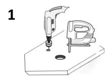
Cut holes if necessary for waste and tap
