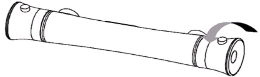
To control the flow of water and to turn on and off, turn the handle on the left, away from the user to increase flow.
