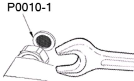
Removal of the mixer from the wall is required, turn off water.
