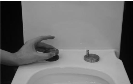
3. Adjust the hinges to a proper distance and place the metal cover onto the hinges
