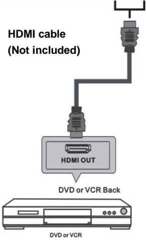
Use HDMI cable to connect the unit with other devices to receive high-definition multimedia signal.
