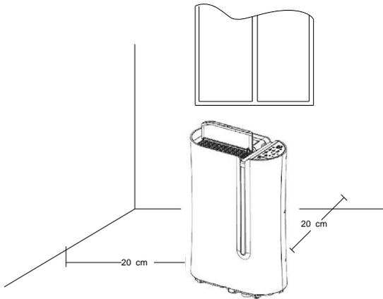
Allow at least 20 cm space around the unit. This dehumidifier is designed only for indoor residential or small office applications and any commercial or industrial use will invalidate the warranty.
