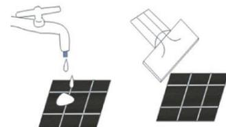
Remove the ABS filter frame. If the optional carbon filters are fitted, remove them from the frame and Hoover gently approximately every 2-3 weeks.
