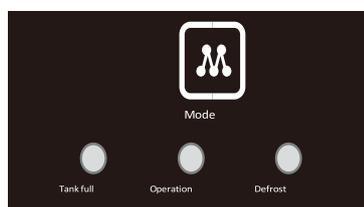
**SMART MODE:** This is designed for maximum convenience and maintains the ideal domestic environment humidity level of 50-55% while saving electricity. This is the default mode and is recommended for most users.
