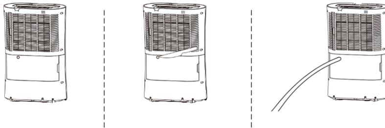
Make sure the connection between pipe and the drain outlet is tight and does not leak. Then direct the pipe to a suitable drainage point. This unit uses gravity to dispose of water hence the drain should be lower than the water outlet on the unit. Put the tank back. Be sure to run the water pipe downward and let the water to flow out smoothly. Do not kink or bend the pipe.
